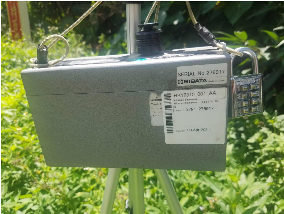
Air quality monitoring equipment (portable dust meter) at DM-5
