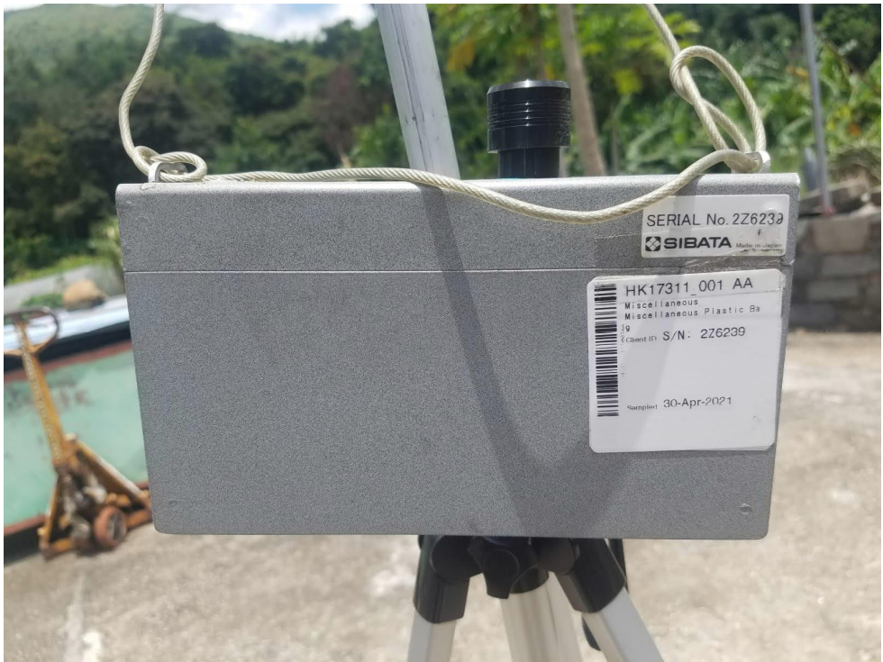
Air quality monitoring equipment (portable dust meter) at DM-6
